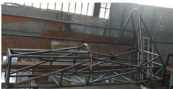
**Figura 2.9** Bastidor Tubular
