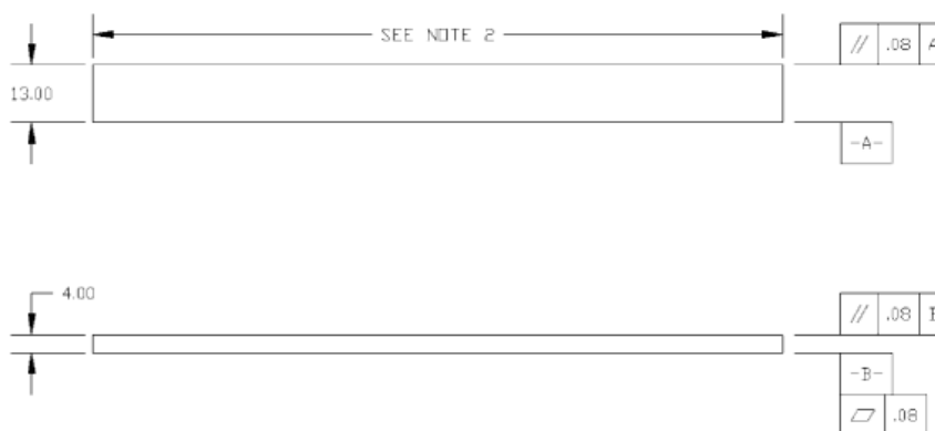
FIG. 4 Standard Flexural Test Specimen Drawing (SI)
