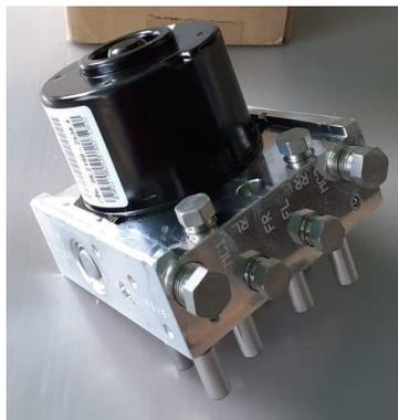
**Figura 1.8 Motor bomba**
