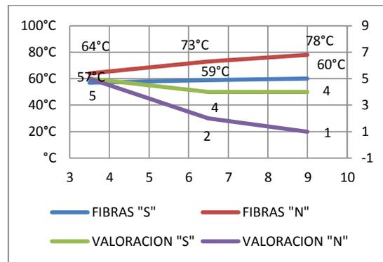
Fig. 14 Chart outlet temperature of the material and assessment of tangled with the speed of the cooling telera
