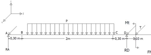
**Picture 1: Diagram of spindle free body.**
