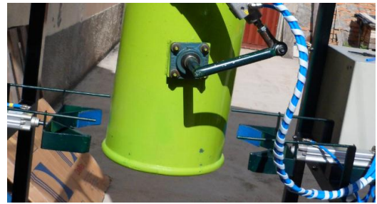
Fig.9 Bag clamping mechanism For performing weight measurement being filled into sacks, the platform is placed in the bottom of the hopper mouth, a distance determined by the dimensions of bags of flour on the market, to perform good counted.
