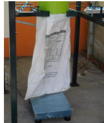
Fig. 10 Mounting weighing platform
