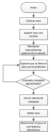
Fig. 1. Diagram manual weighing and filling sacks of flour 50 kg
