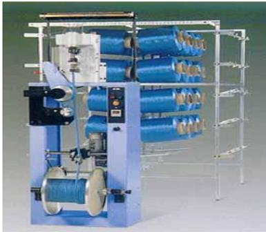
After making the cones of the same color are placed on a wooden frame, and each wire strand passes through a brush for separating the strands.
