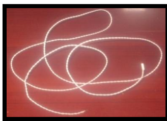
Figura 47. Termistor MA100GG103A NTC
