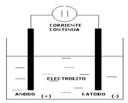
When an electric current flows through the electrolyte, ions move in the solution. The anions are directed towards the anode and captions toward the cathode. One of the chemical compounds most frequently used in dyeing of cellulosic fibers, is the sodium chloride (NaCl). The electrolysis of molten sodium chloride is:
