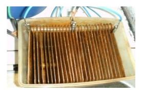
The electrodes have the following dimensions: 15.1 cm long at the base and 15.8 cm long at the top, with a height of 13.2 cm. In the middle part of the base has a semicircle shaped groove with a diameter of 2.3 cm, which is designed to give accommodation to the cylinder feeder the effluent by treat, in a base end is located an orifice of 0.75 cm equal diameter and a perpendicular at the top,
