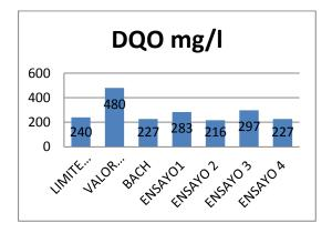
Comparative trials regarding Chart 27. removal of COD Standard. The first bar shows the maximum allowable level, the second indicates the location of the effluent prior submission to to electrocoagulation, the third bar indicates the level of debugging with a longer residence of the effluent, concluding that rotates once a colloidal phase load polluting, has no additional positive result. The assay two four
