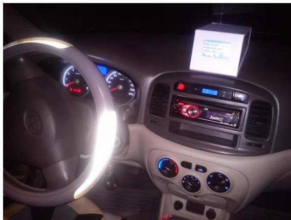
Fig.2 Digital taximeter was installed in a Hyundai Accent 2010 car with digital odometer.
