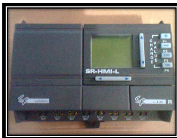
Figura 3-8 PLC 22MRDC de Array Electronic.
