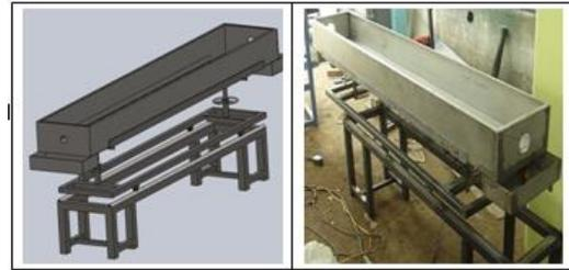
Figures 17. I design and construction of cooling tub.
