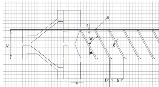
Figures 20. Section of the screw and mold general data.
