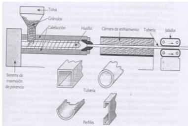
Figure 3. Equipment for extrusion profiles.
