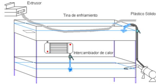
Figure 12 Cooling System Water recirculation.
