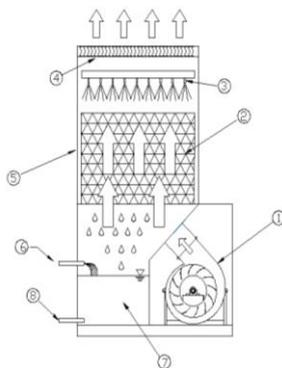
Figures 16. Parts of a cooling tower.
