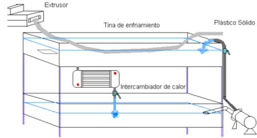
Figure 12 Cooling System Water recirculation.
