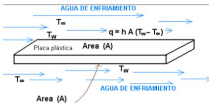
Figure 13 plastic pallet where the face is in Z which emits more heat, because there is greater area
