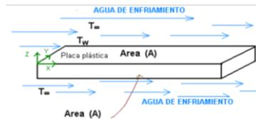
Figure 13 plastic pallet where the face is in z which emits more heat, because there is greater area
