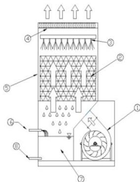
Figures 16. Parts of a cooling tower.
