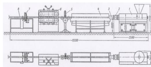
Figure 10. Installation for extruding tubes of thermoplastic material with a 60mm diameter screw.
