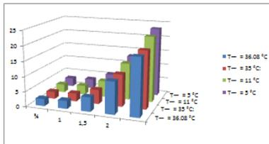
**Figures 22.** Representation of the heat that transfers the tube of plastic toward the water.
