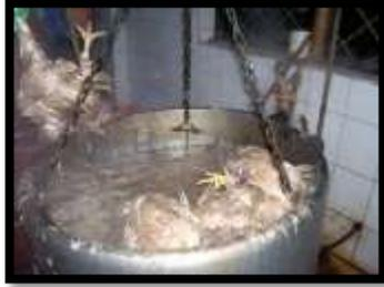
The temperature and scalding time are parameters that should be monitored and controlled to achieve the proper feather loosening to avoid overheating that generates the birds cooking. The temperature in which scalding is performed without any complications reaches up to 54 degrees Celsius. Scalding time usually takes 2—3 minutes, depending on the animal's characteristics.
