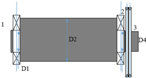
**Figure 9.** Diagram of the different diameters of the shaft
