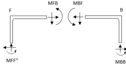
**Figure 4.** Balancing of moments in the gaskets I and K
