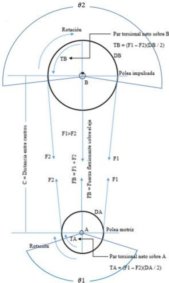
**Figure 8.** Diagram of forces in the drive and driven pulleys
