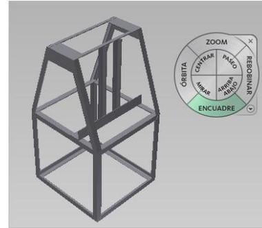
**Figure 13:** Machine frame designed in CAD Inventor Professional
