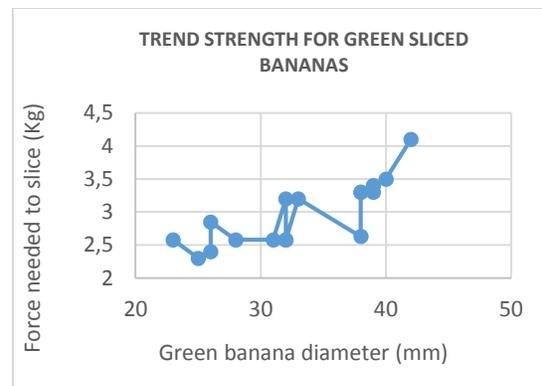
**Figure.4.** Diameters of green bananas and necessary force for cutting
