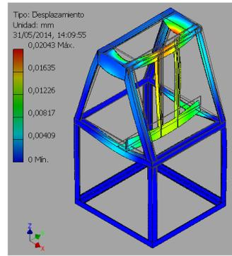
**Figure. 16.** Displacement of the structure
