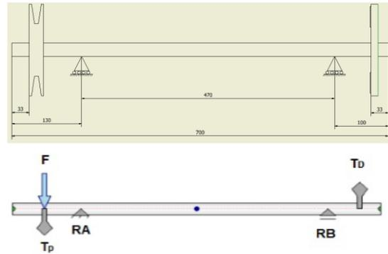
**Figure. 9.** Free body diagram of the shaft.
