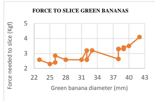
**Figure. 17.** Force required to sliced green bananas
