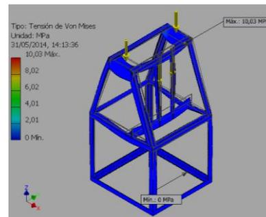
**Figure. 17.** Von Mises stress of the structure
