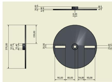
**Figure 6.** Dimensions of the blade.
