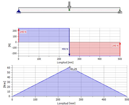
**Figure14:** Diagram Cortes and moments of the beam
