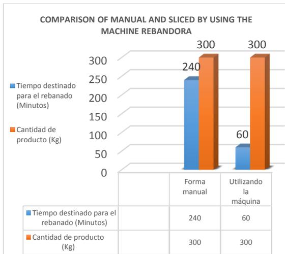
**Figura. 19.** Manual comparison slicer and using the slicing machine
