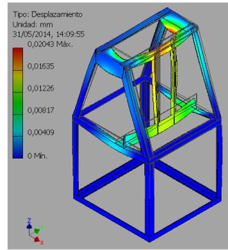
**Figure. 16.** Displacement of the structure
