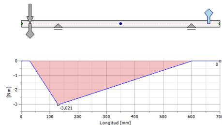
**Figure. 113.** Flector Moment diagram in the plane Y-Z
