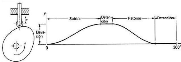
**Figure 15. Displacement diagram of cam and follower**
