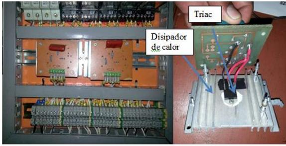
**Figure 12. Horizontal sealing Power Board**
