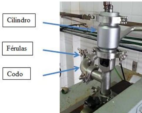
**Figure 1. Cylinder feeder**
