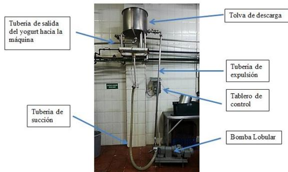
**Figure 19. Assembly of the elements of the level Control System**
