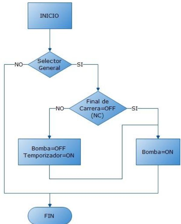
**Figure 18. Flowchart of the level Control**
