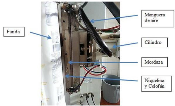
**Figure 5. Elements of sealing vertical**
