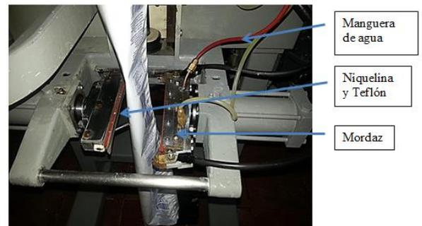
**Figure 6. The Horizontal sealing elements**
