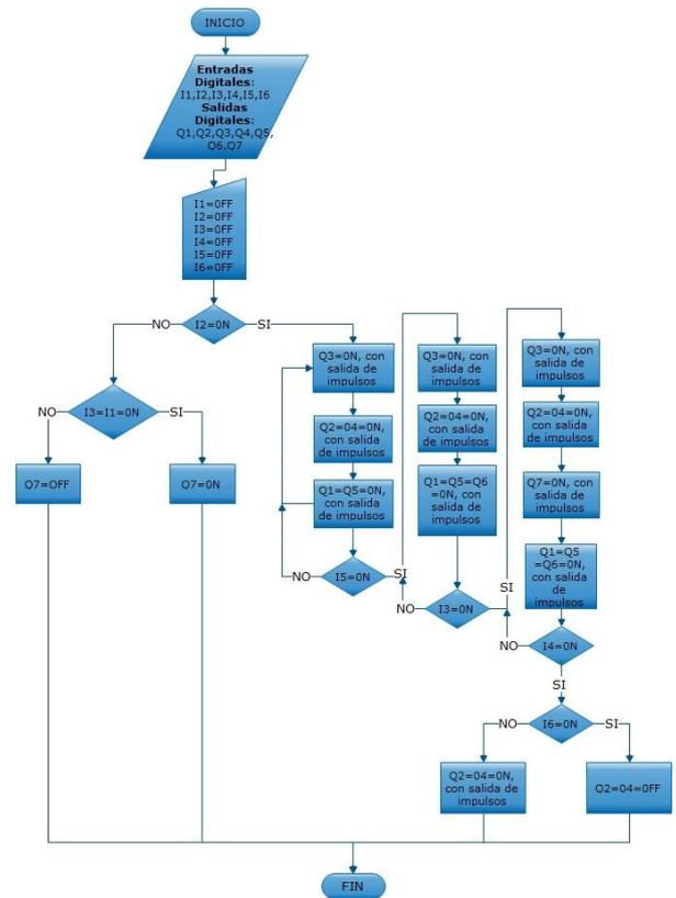
**Figure 17. Flowchart of the automatic system of the machine**
