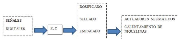
**Figure 9. Block diagram of the general system**
