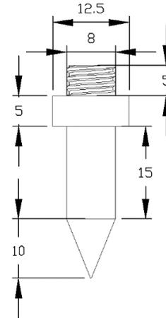
**Figure 6.** Suction in mm nozzle
