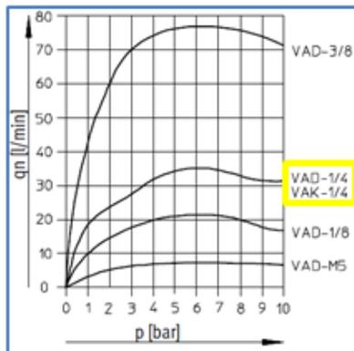
**Figure 20.** Behavior of generators vacuum VAD and VAK depending on the suction capacity and working pressure
