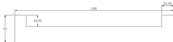
**Figure 1.** Front suction manifold [mm]
