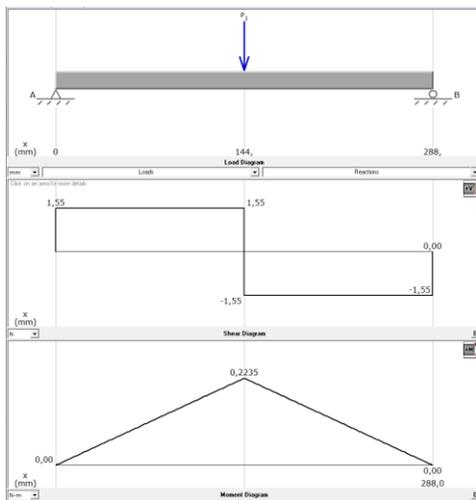
**Figure 8.** Diagram of cuts and moments of shaft
