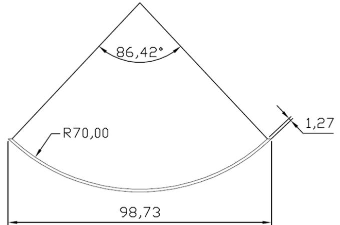
**Figure 11.** Radius of arc of the basis of seeds in [mm]
