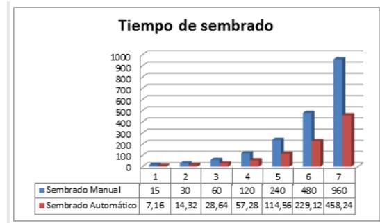
**Figure 52** Production of seedlings with a seeded manual and automatic
