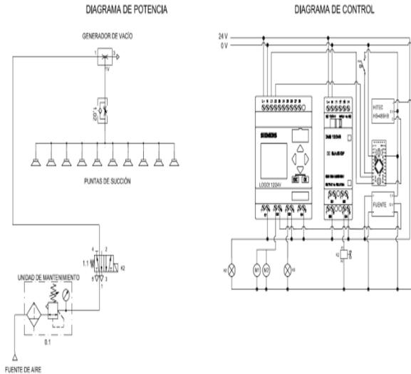
Figure 37. Pneumatic connection diagram
