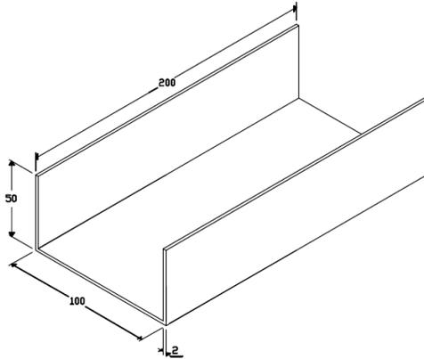
**Figure 17.** Structure for the sower of seeds in [mm]
