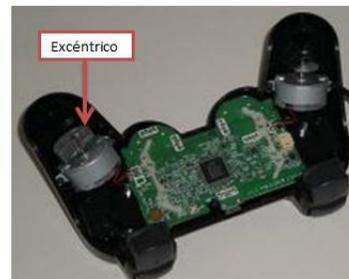
**Figure 30.** Engines eccentric lever Play Station
