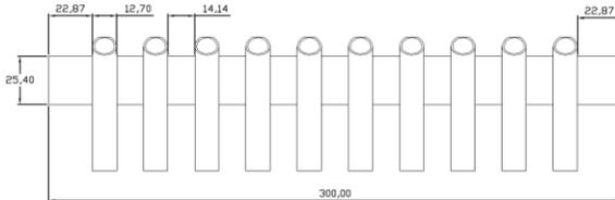
**Figure 14.** Distributor of seeds in [mm]
