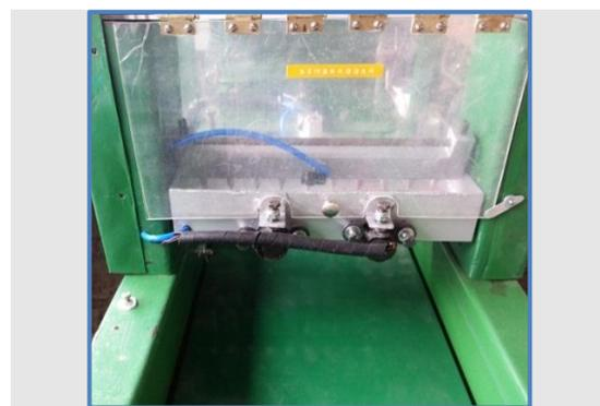
**Figure 53.** Protection of the seed drill machine acrylic
