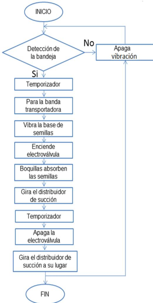
**Figure 35.** Flowchart of the PLC
