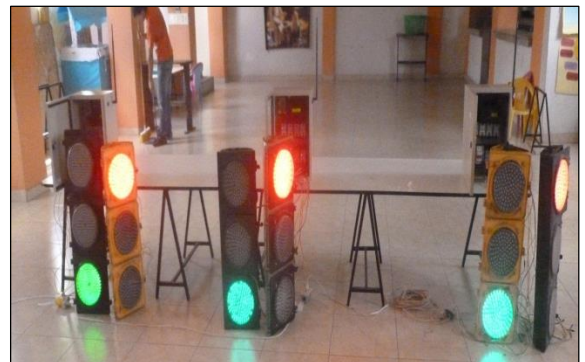
Figure 15. Junctions system working in Normal mode
