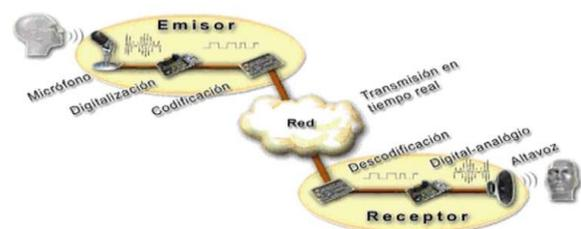
Figure 1. Voice transmission in digital networks.
