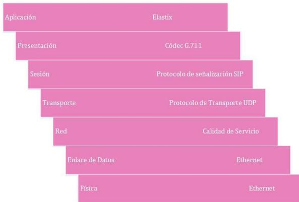
**Figure 6.** IP Telephony in the UTN within the OSI model.
