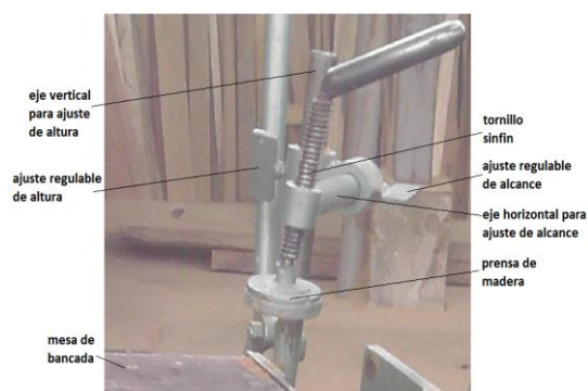
Figure 4. Mecanismo for pressing the wood.
