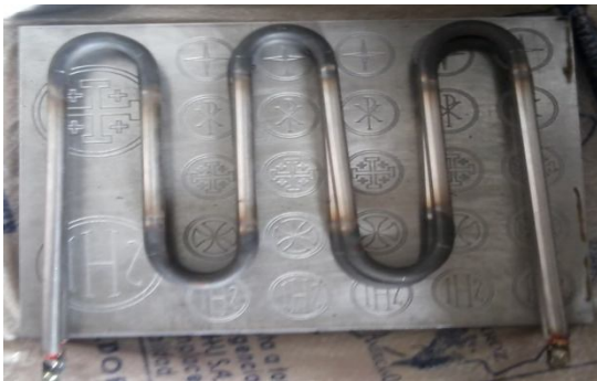
FIGURE 7. Design of the electrical resistances
