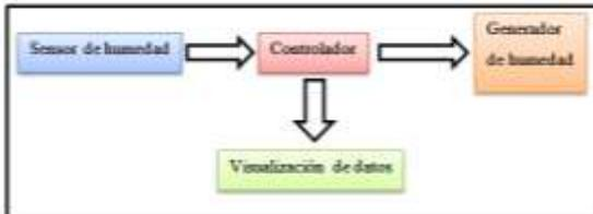
The control system is designed according to the needs of the application means. For data acquisition and process control moisture generation is needed:
