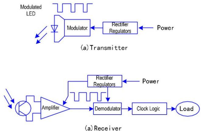
Figure 5. Infrared sensor operation.
