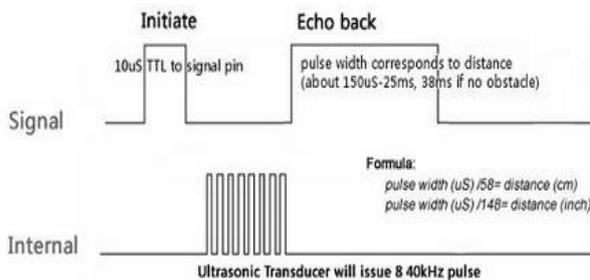
Figure 3. Ultrasonic sensor operation.
