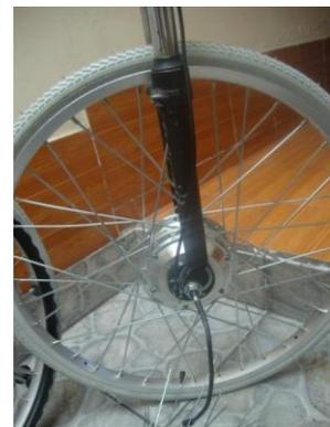
Figure 8. Brushless motor coupled to the wheelchair rim.
