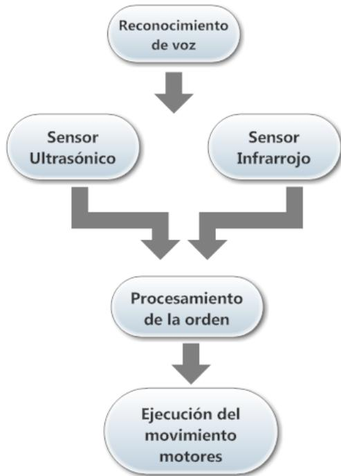
Figure 1. System blocks diagram.
