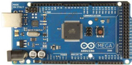
**Figure 6.** Arduino Mega 2560
