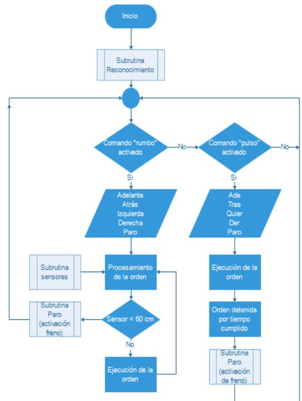
Figure 11. Basic system flowchart
