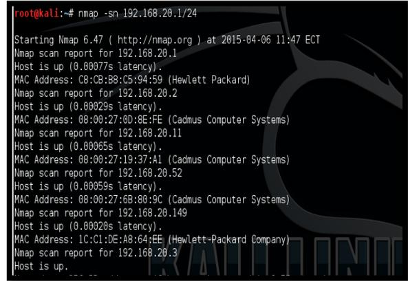
Figure 13. Scan of host through Nmap
