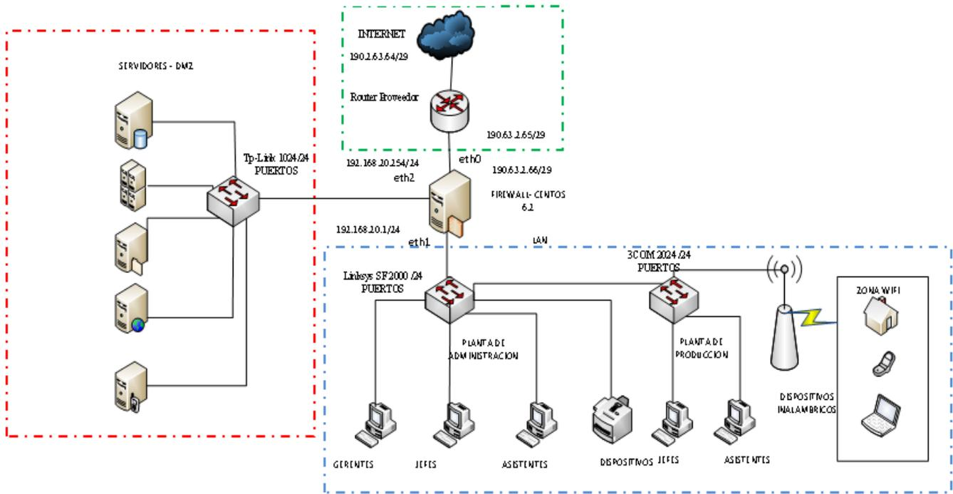
Figure 9. Design of network topology
