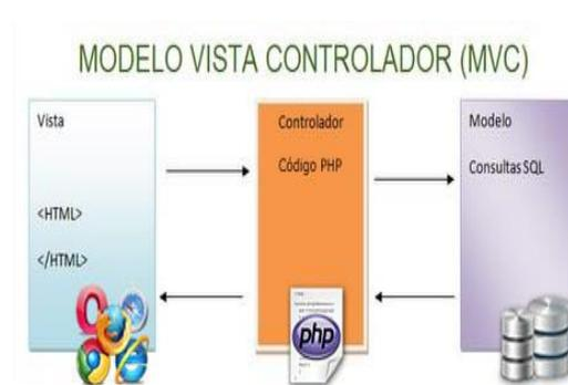
The model is in charge of data management and makes queries to the data source either a database or a data file. Only the driver can interact with the model and through a function that will return or take data but it cannot change the model performance.
