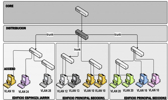
Fig. 41. Segmentation of the network under a hierarchical model. Source: <http://sistemasumma.com/2012/02/19/redes-jerarquicas/>
