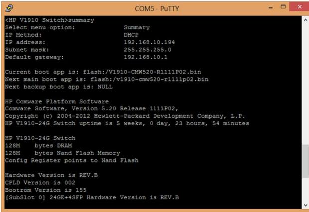
Fig. 26. Access to the console switch HP-1910.
