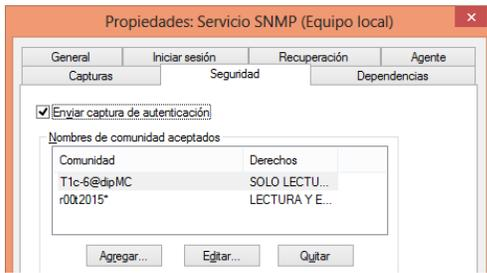
Fig. 15. Enabling SNMP protocol. Source: Operating system Windows 7.
