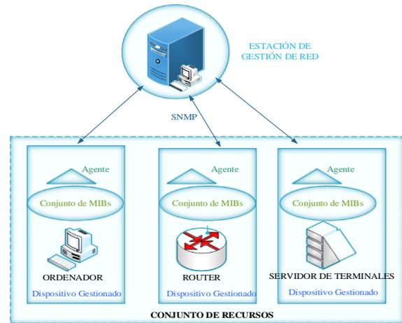
Fig. 3. SNMP management architecture.
