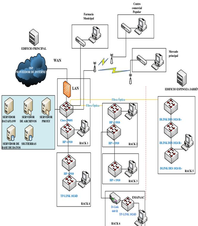
Fig. 7. Topology logic of the LAN GADIPMC.
