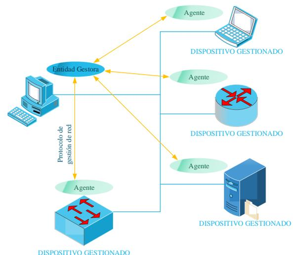
Fig. 1. Elements of a network management system
