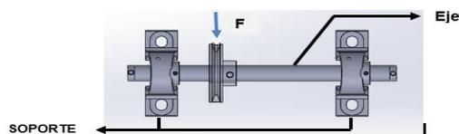
Figure 3.2. Axle bearings.
