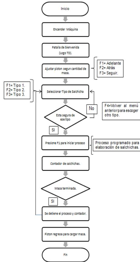
Figure 4.1. Schematic flow chart control.
