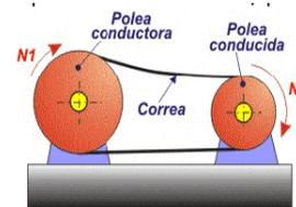
**Figure 3.1.** Pulley belt drive system. Source. (Technology, 2007)
