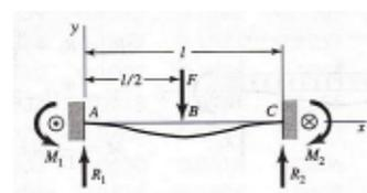
**Figure 3.6** Beam A- B (model with central charge fixed supports)
