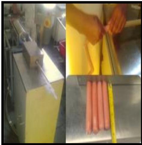
**Figure 5.6** Process formed (twister machine sausage).
