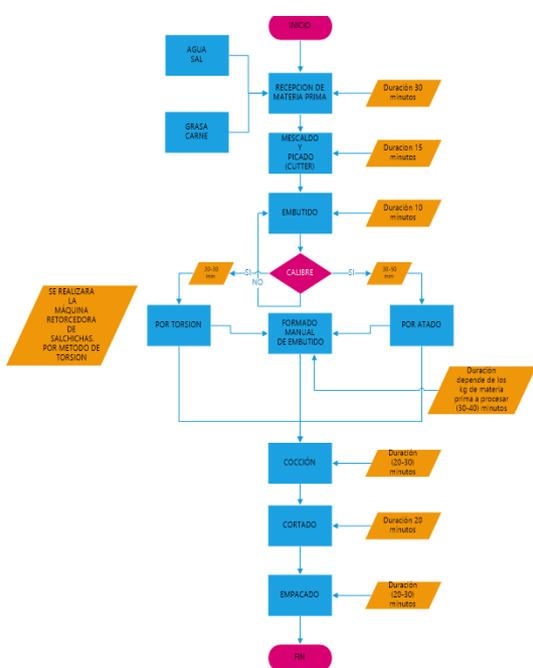
**Figure 1.1.** Manual twisting process .
