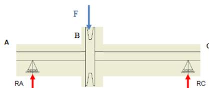
Figure 3.3. Free-Body diagram
