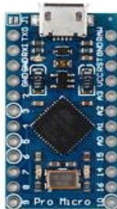
**FIGURA 17:** Arduino Pro Micro
