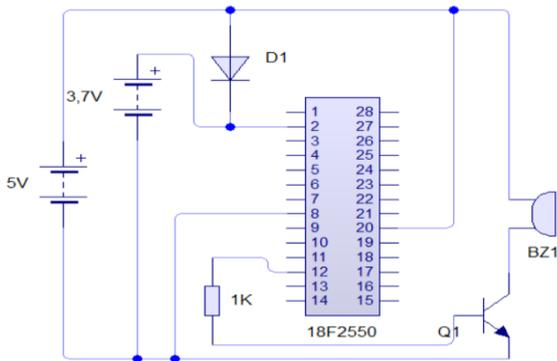
**Figure 5** System Diagram battery charge
