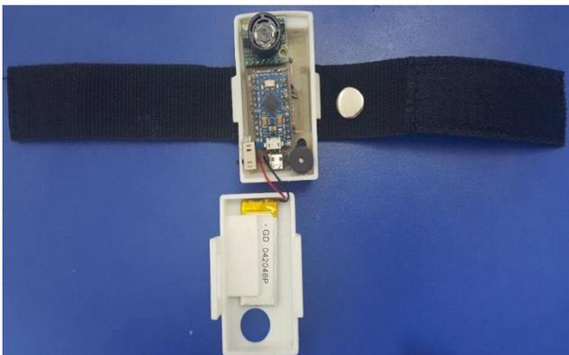
**Figure 25** Photo housings handles with plate and battery
