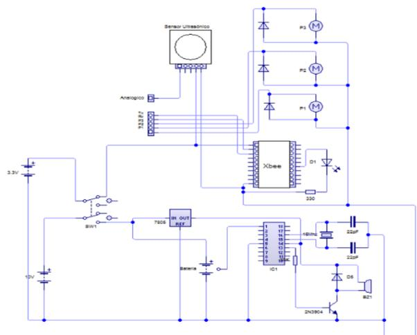
Figure 13 complete electronic circuit diagram belt
