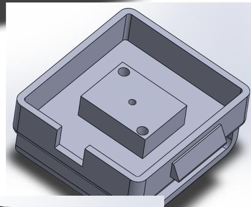
**Figure 23** lower housing front sensor
