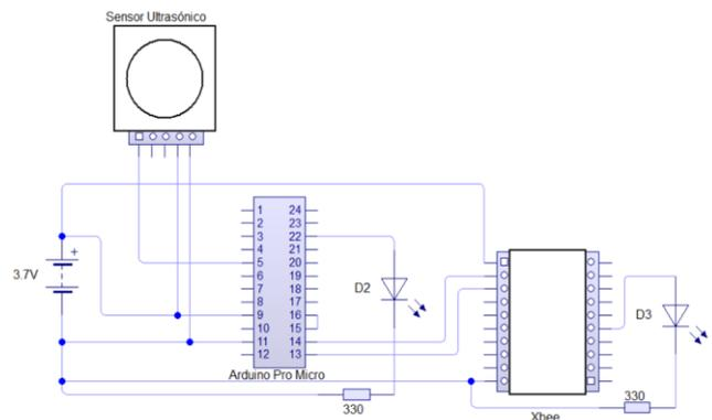
**Figure 4** Diagram main circuit handle
