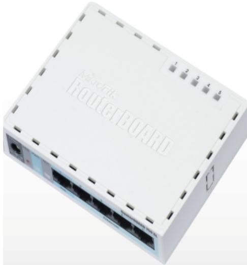
The RB750GL is a small SOHO router in a white plastic case. It has five independent Gigabit Ethernet ports and optional switch chip functionality for wire speed Gigabit throughput.
