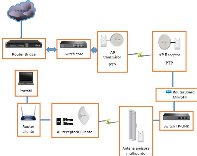
Fig 9. General structure of the network
