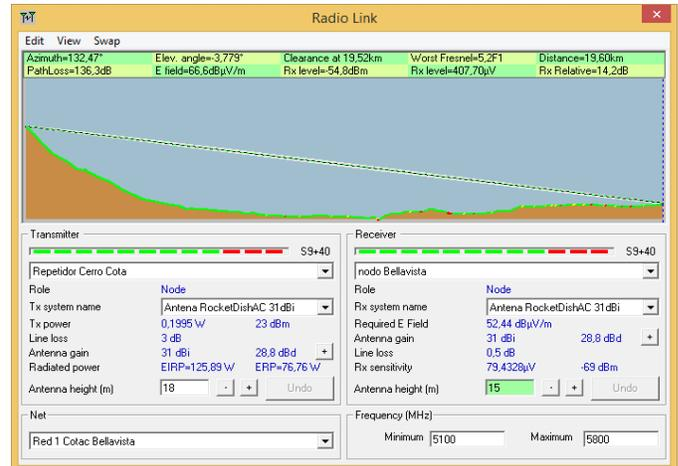
Fig 13. Profile of the link between Cerro Cotacachi-Bellavista
