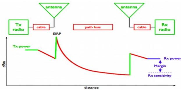
Fig 11. Basic Wireless Communication System
