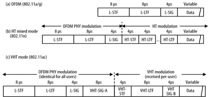
Fig 1. VHT Physical Layer Frame Format
