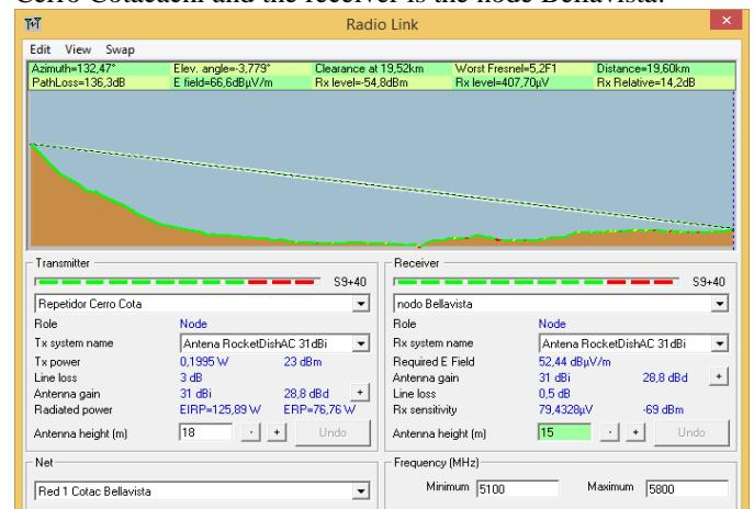
Fig 13. Profile of the link between Cerro Cotacachi-Bellavista
