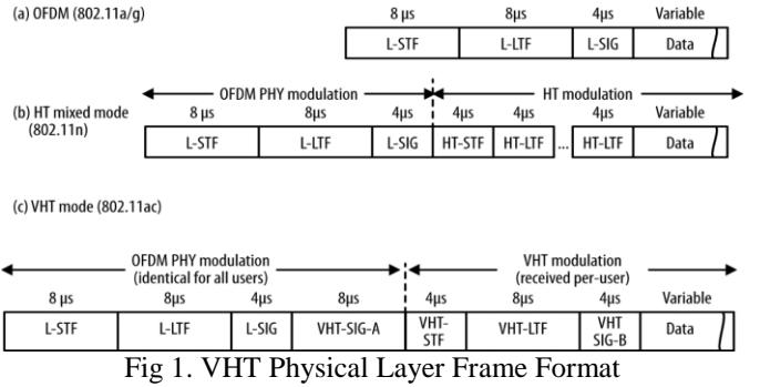
Fig 1. VHT Physical Layer Frame Format
