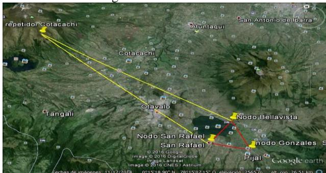
Fig 7. Interconnection of the primary backbone network
