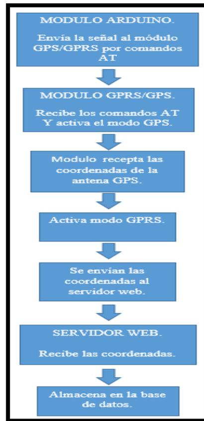
Figure 33. Diagram of operation of GPS and GPRS.
