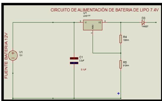
Figure 29. Battery power circuit.
