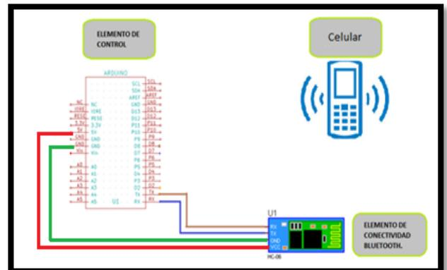
Figure 23. Bluetooth connection circuit.
