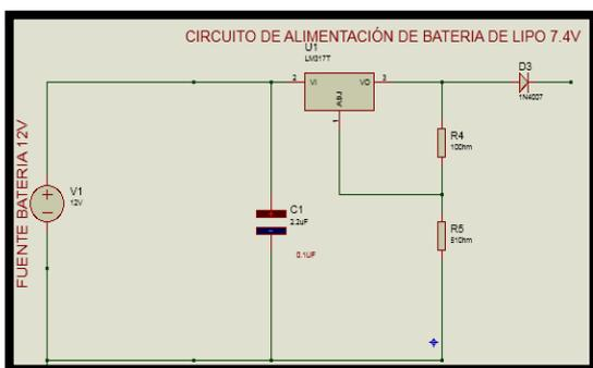
Figure 29. Battery power circuit.
