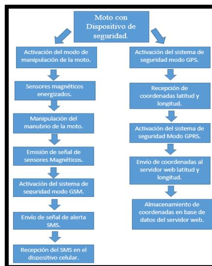
Figure 17. Diagram of operation of the security system.
