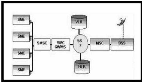
Figure 10. SMS network architecture.
