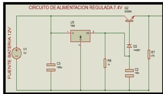
Figure 28. Regulated power supply circuit.
