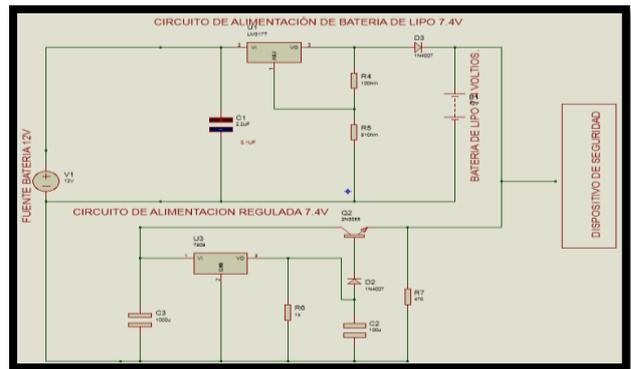
Figure 30. Power supply circuit.
