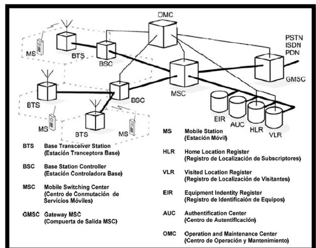
Figure 9. Architecture GSM.
