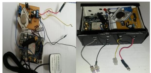
Figure 46. Case of the safety device.
