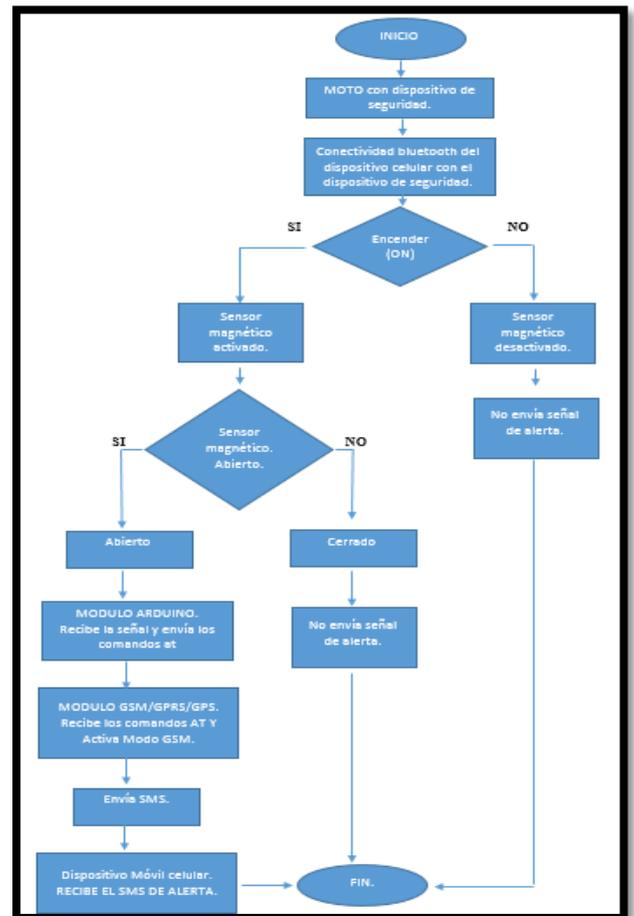
Figure 32. Flowchart of the security system.
