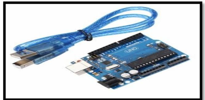
Figure 7. Micro controller ARDUINO.
