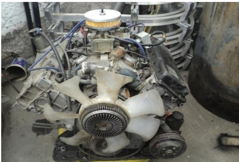
**FIGURA 19.** Motor a carburador V6.
