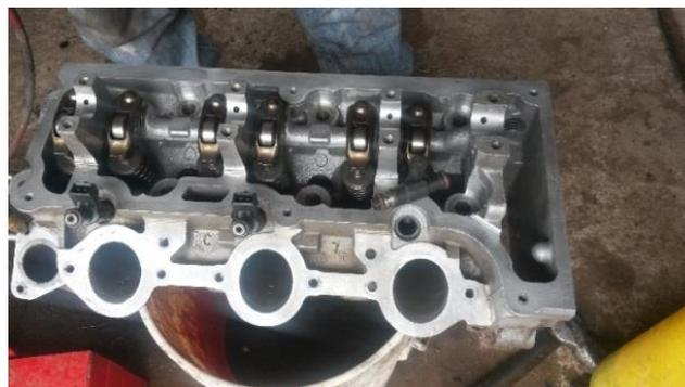
FIGURA 64: Culata motor Ford Explorer 4.0L.
