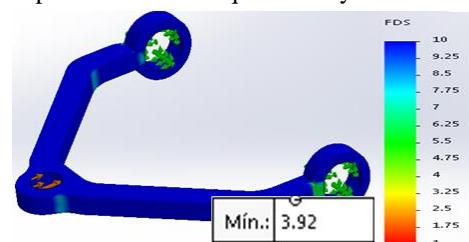
Figure 11. Safety factor on the front top suspension table
