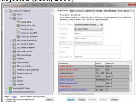
Figure 8. Application of material.
