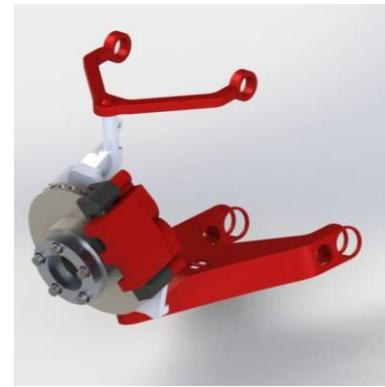
**Figure. 6.** Front suspension.
