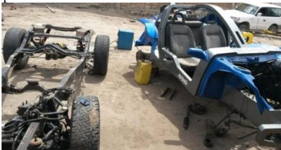
**Figura13.** Chassis and body of the vehicle Peugeot 604 type Buggy.
