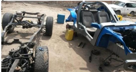
**Figure 13.** Chassis and body of the vehicle Peugeot 604 type Buggy.
