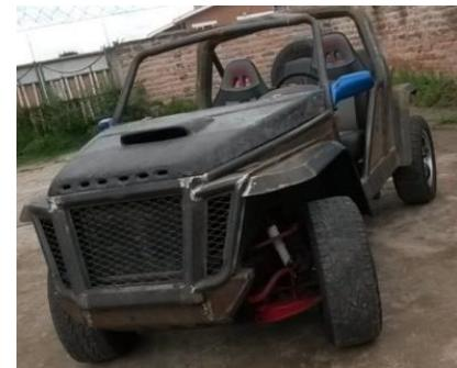
**Figure 18.** Finished body assembled to the chassis.
