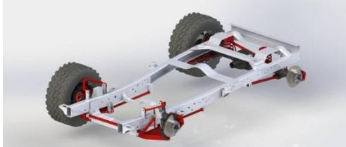
**Figure 12.** General assembly of the chassis and its components.
