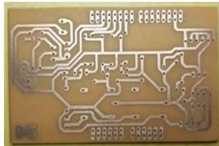
Fig. 10. Circuit board design of the Shield Interface board.
