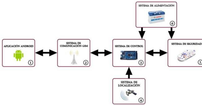
Fig. 1. General block diagram of the Vehicle Location and Safety System prototype.
