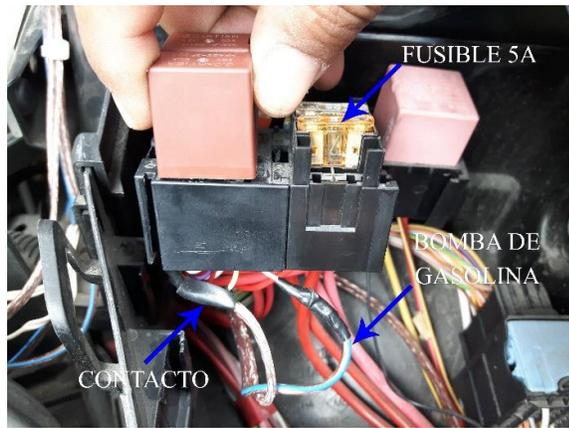
Fig. 29. Connection of the petrol pump and vehicle contact signals.
