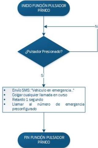
Fig. 9. Panic button flow diagram.
