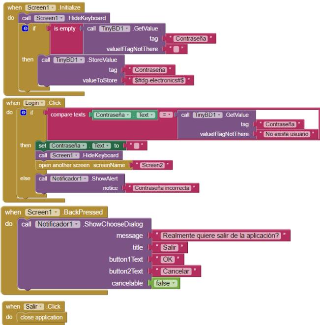
Fig. 21. Block Programming of the Login Screen.
