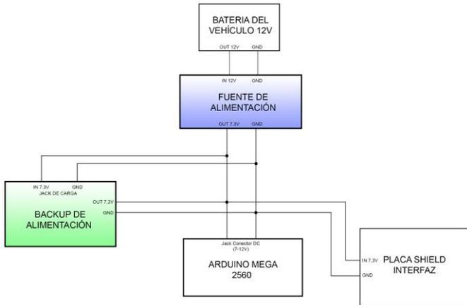
Fig. 14. Block Diagram of the Power system.
