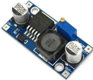
Fig. 15. LM2596s voltage regulator module.
