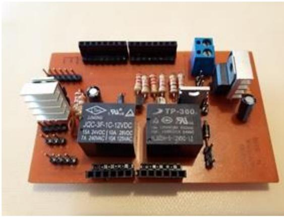
Fig. 24. Shield Interface Board.
