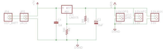
Fig. 5. Electrical diagram of the 3.3V voltage regulator circuit.
