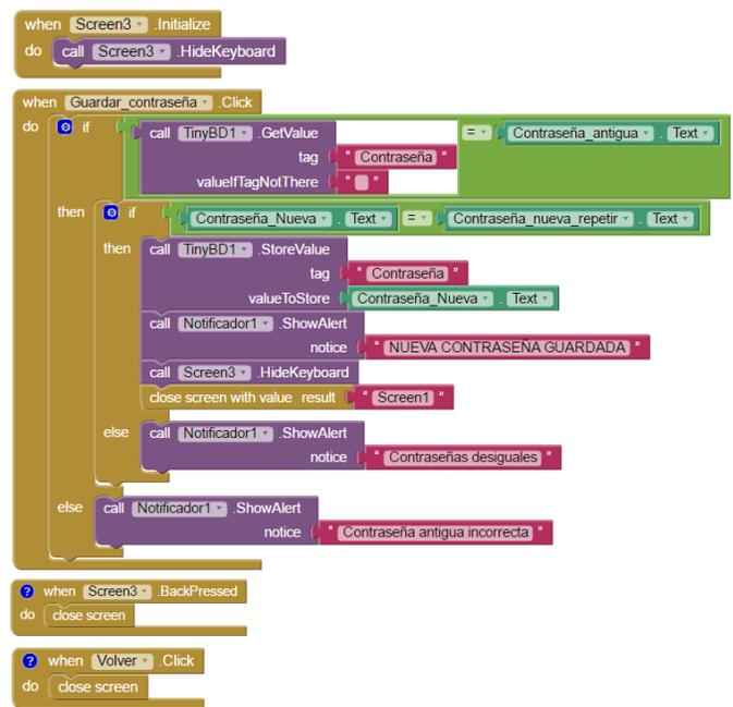
Fig. 23. Block programming of the Configuration Screen.
