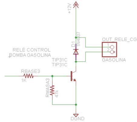
Fig. 7. Relay control circuit using an NPN transistor TIP31C.
