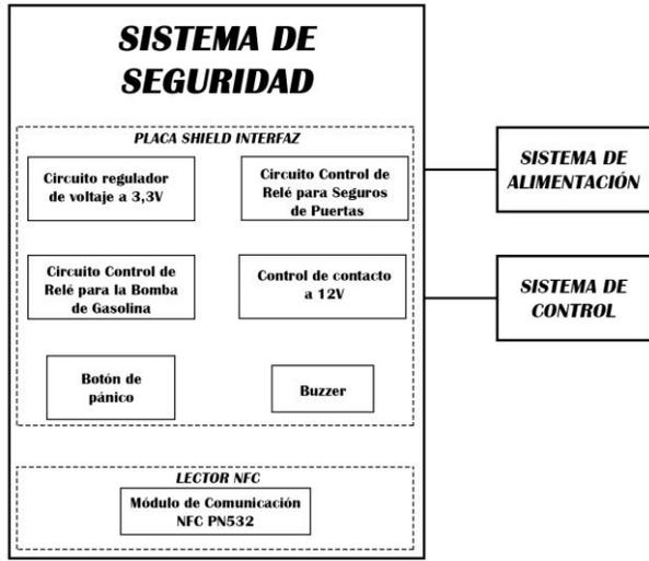
Fig. 3. Block diagram of the Security System.
