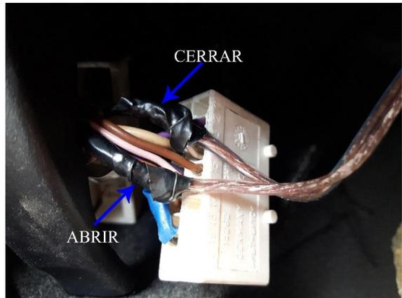
Fig. 28. Connection of the central locking signals.
