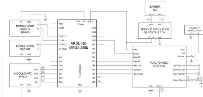
Fig. 17. General electrical diagram of the vehicle location and safety system prototype.
