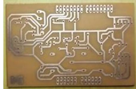
Fig. 10. Circuit board design of the Shield Interface board.
