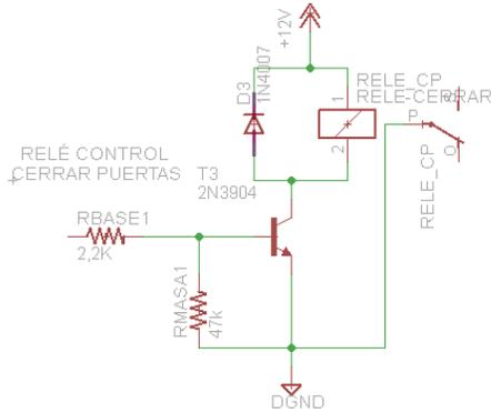
Fig. 6. Relay control circuit for vehicle door locks.
