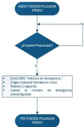
Fig. 9. Panic button flow diagram.
