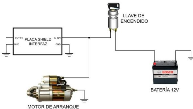
Fig. 8. Connection diagram of the vehicle ignition circuit to the Shield interface board.
