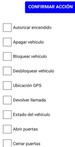
Fig. 30. Interface of the screen of actions of the Android application.
