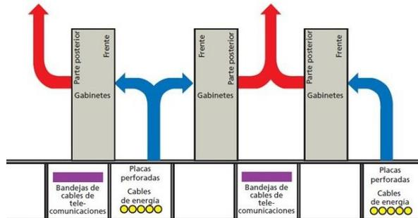
Figure 3. Example of distribution of hot and cold aisles
