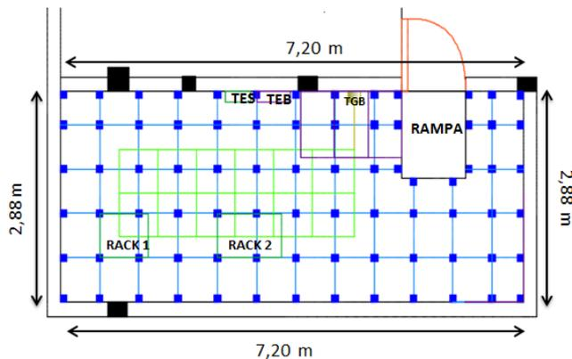
Figure 16. Grounding mesh
