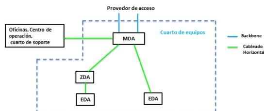
Figure 1. Reduced topology of a Data center
