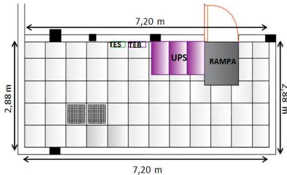
Figure 14. Location of electrical boards and UPS
