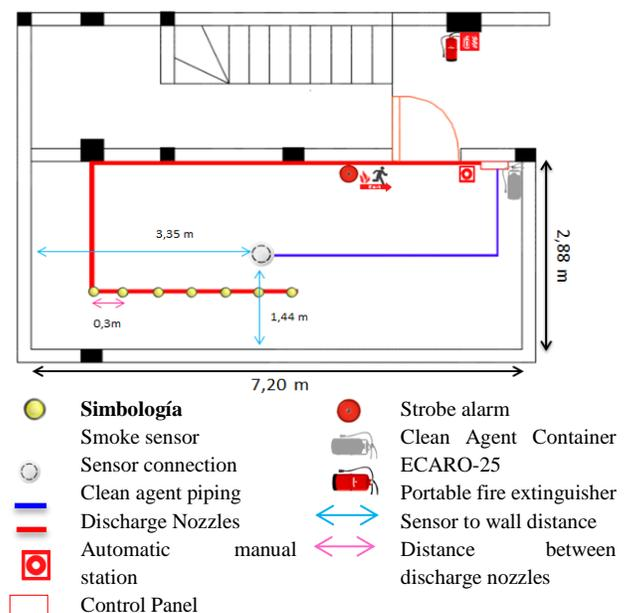
Figure 19. Schematic of the fire detection system
