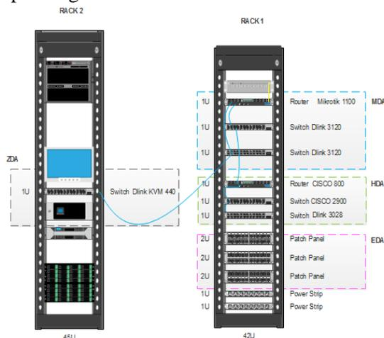
Figure 5. Diagram of distribution of the equipments with their corresponding zones
