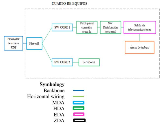
Figure 4. Connection diagram of the telecommunications System
