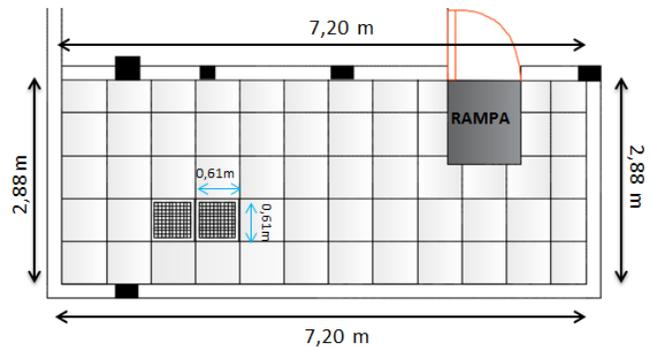
Figure 135. Placement of tiles on transoms
