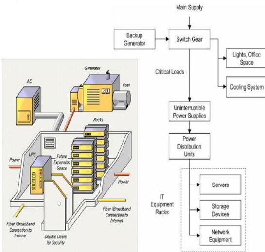
Figure 2. Electrical System Connections
