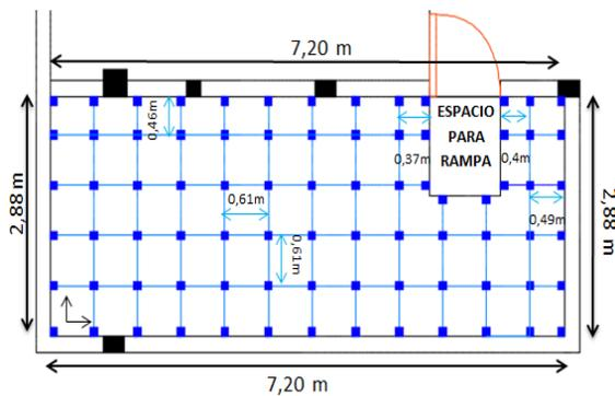
Figure 12. Installation of pedestals and crosspieces
