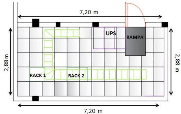
Figure 16. Ladder Location for Electrical Wiring
