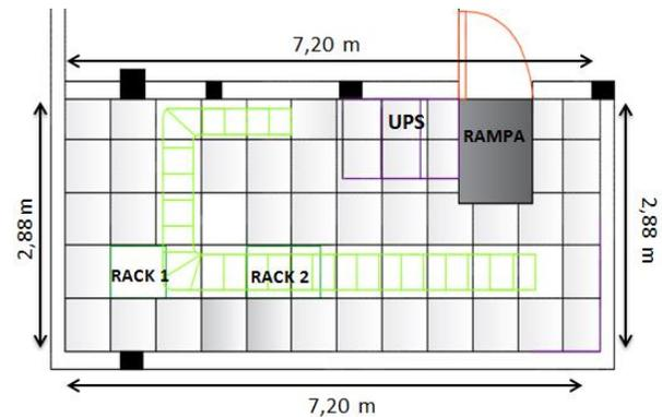
Figure 16. Ladder Location for Electrical Wiring
