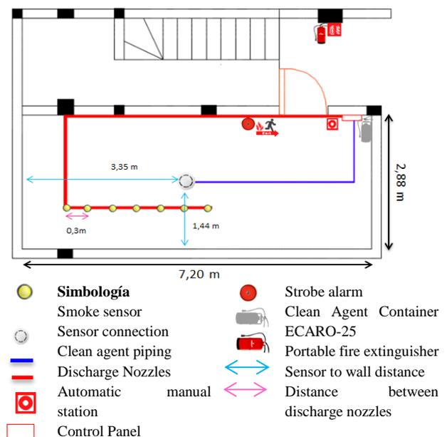
Figure 19. Schematic of the fire detection system
