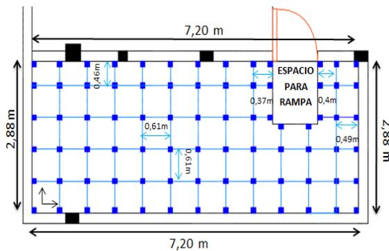
Figure 12. Installation of pedestals and crosspieces
