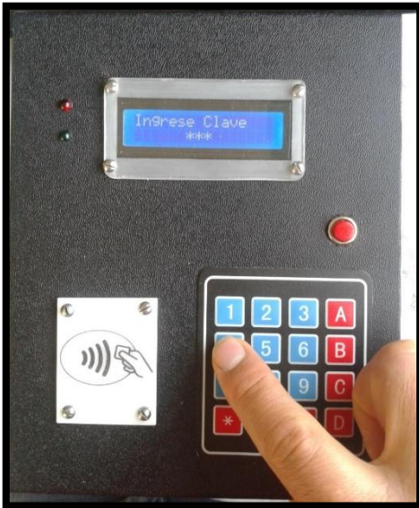
Fig. 17 Activation of subroutine for keyboard input.
