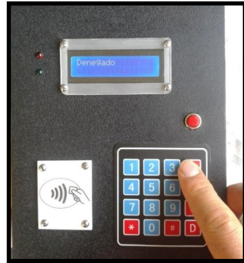
Fig. 19: Incorrect key entry using matrix keyboard.
