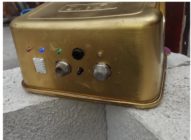
Figure 18. Prototype of the multisensor system warning of a fire. Source: Project development.
