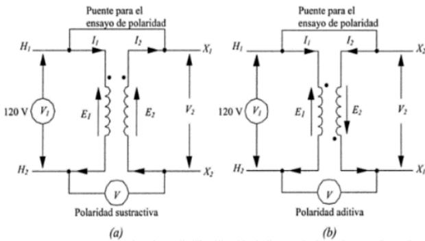
Fig. 3 Transformer Polarity
