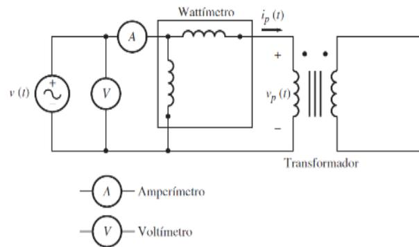
Fig. 1 Open circuit test
