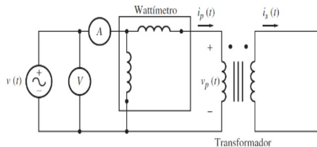
Fig. 2 Short circuit test
