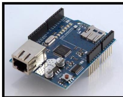
Figura 17. Arduino Ethernet Shield
