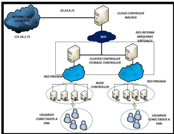
**Figure 6.** Internal Architecture of Eucalyptus and their respective components
