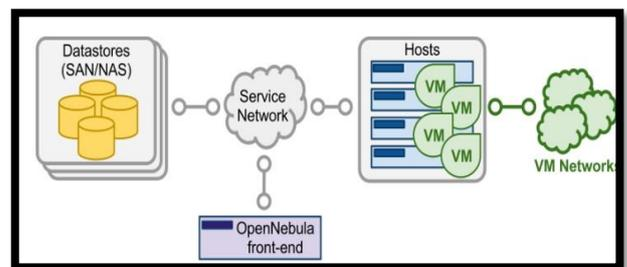
**Figure 7.** Functional Architecture Reference OpenNebula:
