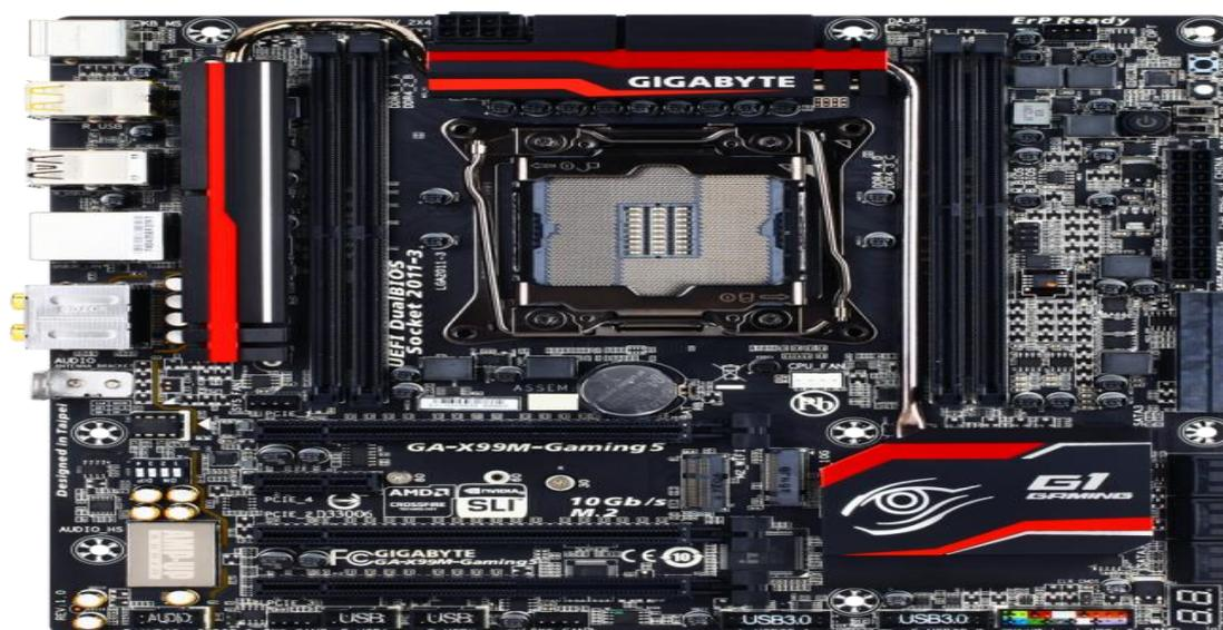
**Figura 6. Motherboard Micro ATX**
