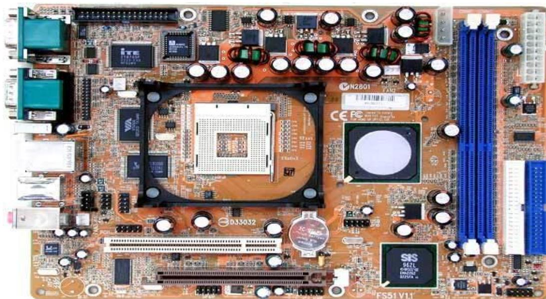
**Figura 7. Motherboard Flex ATX**
