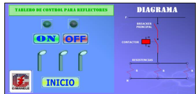
Figure 4. Control of reflectors. MOVICON 11.5
