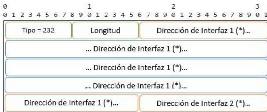
Figura 16. IPv6 Interface Address TLV
