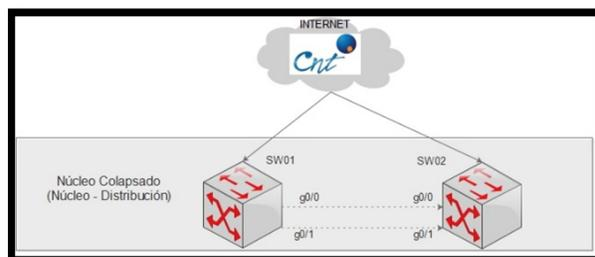
Figure 19. Hierarchical model - collapsed core
