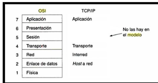
Figure 2. Reference models TCP / IP
