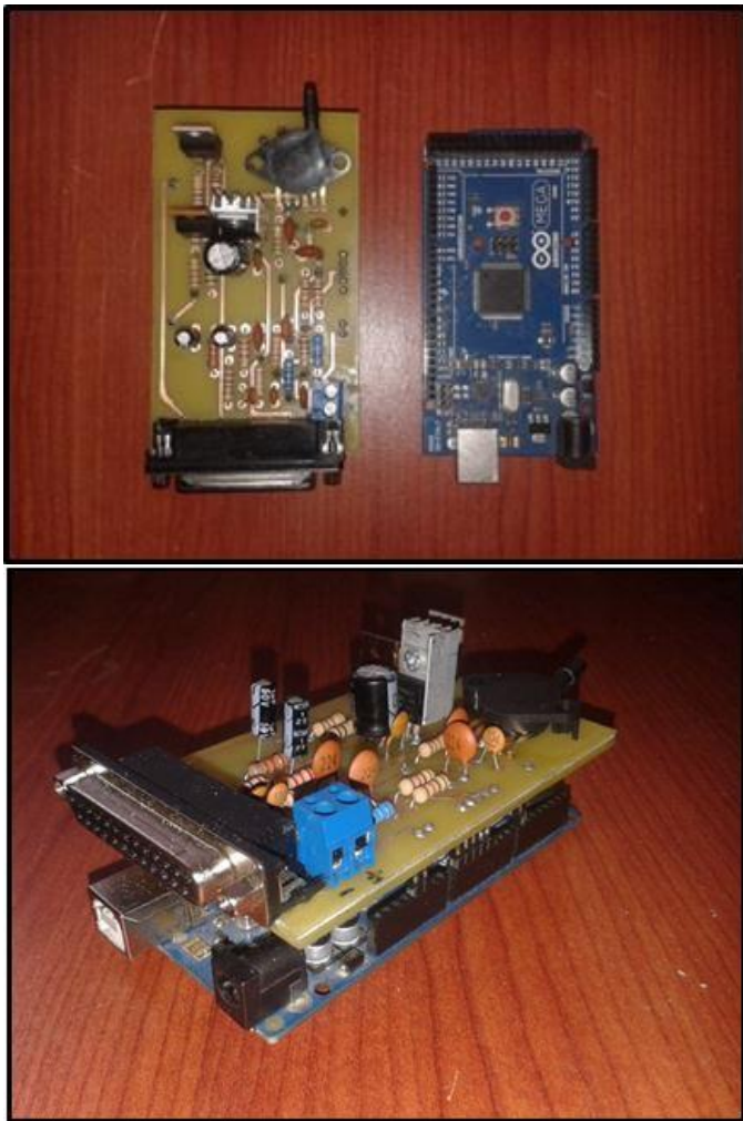
Fig. 10. Electronic control unit.
