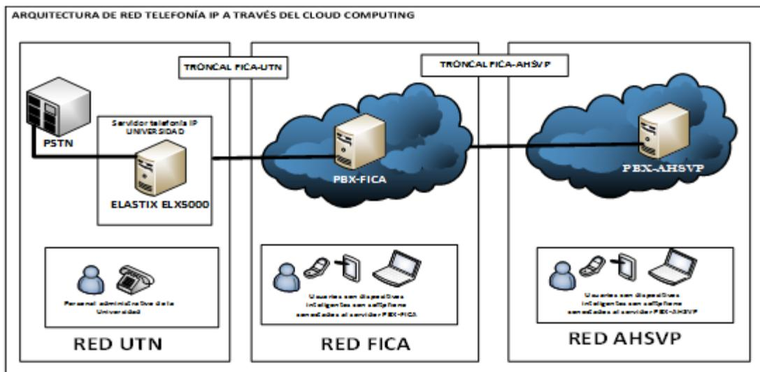
Figure 3. IP telephony architecture in the cloud
