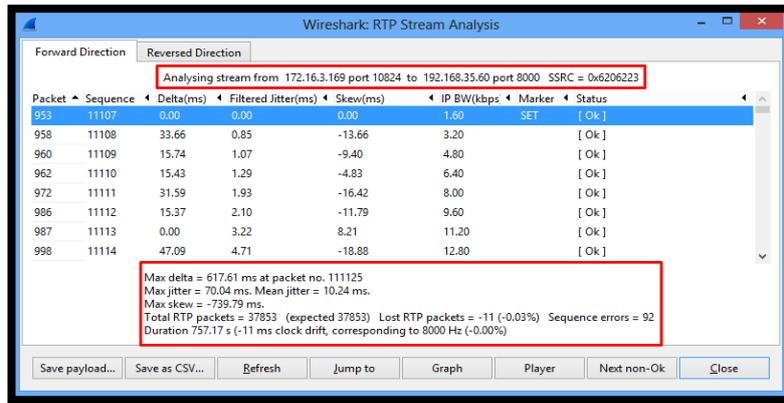
**Figure 8.** RTP traffic capture with Wireshark local level test
