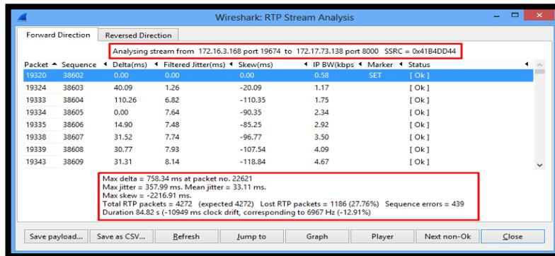
**Figure 9.** Analysis of an RTP packet FICA captured between PBX and PBX-server-AHSVP
