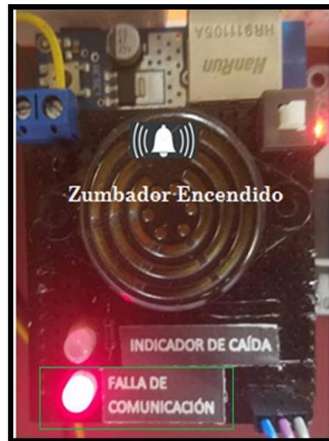
Figure 12: Alarm the failure the communication auditory and visual.
