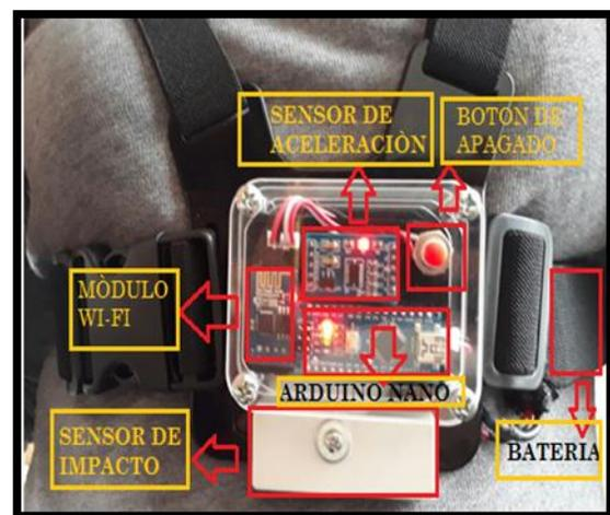
Figure 5. Design end the *módulo sensor*
