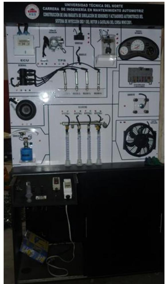
Figure 1 Model of complete simulation.
