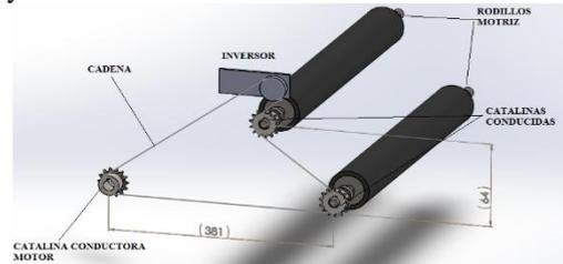
**Figure 18: Transmission system via chain.**
