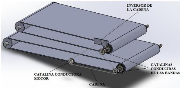
Figure 11: Power Transmission.
