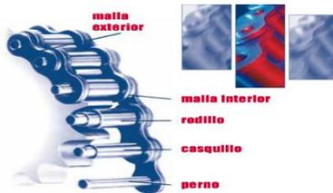
**Figure 15: Main parts of a roller chain**
