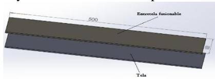
Figure 8: Dimensions fabric and interlining.
