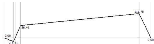
Figure 26: Diagram plane bending moment XZ- drive roller shaft.
