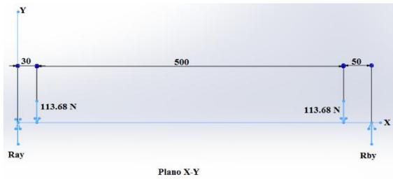
Figure 21: Forces in the X-Y plane.
