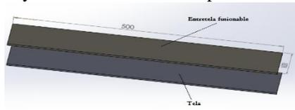
Figure 8: Dimensions fabric and interlining.
