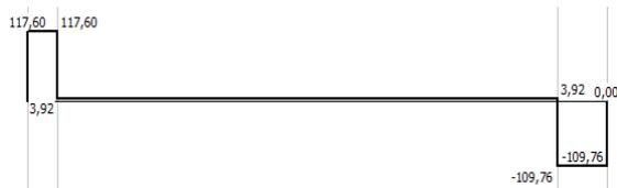
Figure 22: Diagram XY plane shear - drive roller shaft
