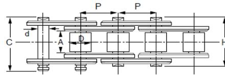
**Figure 17: Main characteristics of roller chain**
