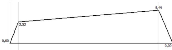
Figure 23: XY plane bending moment diagram - drive roller shaft
