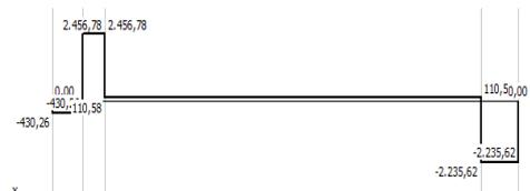
Figure 25: Diagram of shear plane XZ- drive roller shaft.
