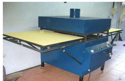
Figure 5: textile Sublimator splicer.
