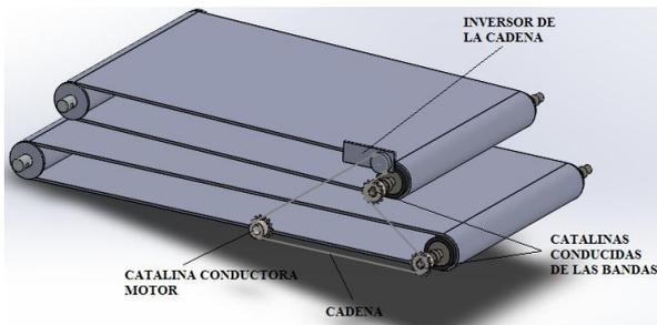
Figure 11: Power Transmission.
